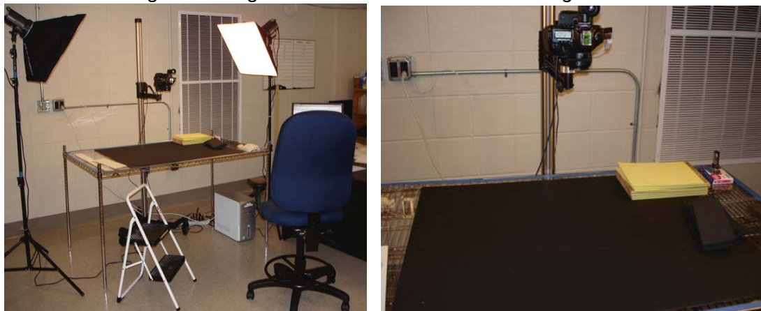
Foldouts are digitized using an overhead camera after book digitization at the Scribe
